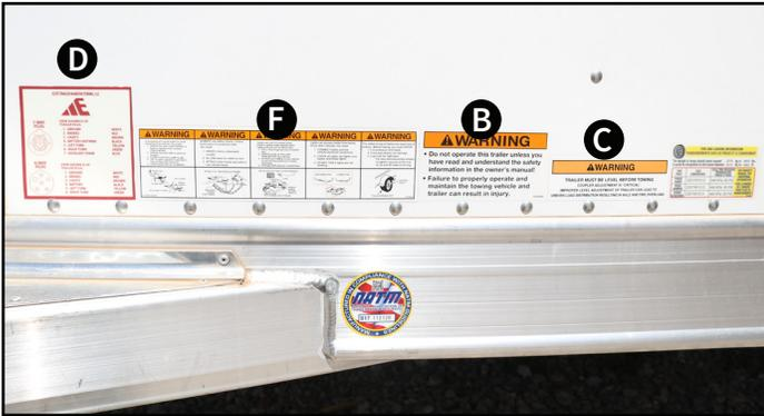
Fig.6 Bumper Pull Safety Warning Labels
