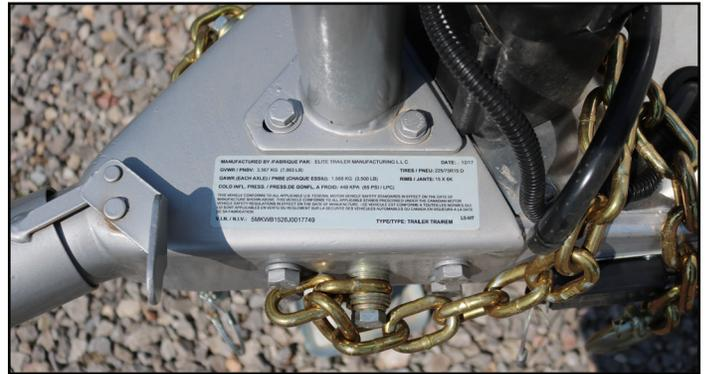
Fig.9 Bumper Pull Trailer VIN Certification Label
