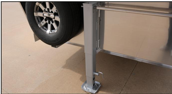
Fig.14 Drop-leg Jack Arrangement
