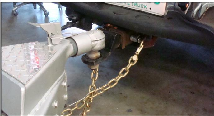
Fig.10 Safety Chain Arrangement
