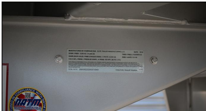
Fig.8 Gooseneck Trailer VIN Certification Label
