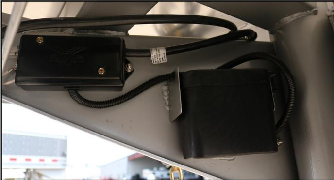
Fig.17 Breakaway Brake System
