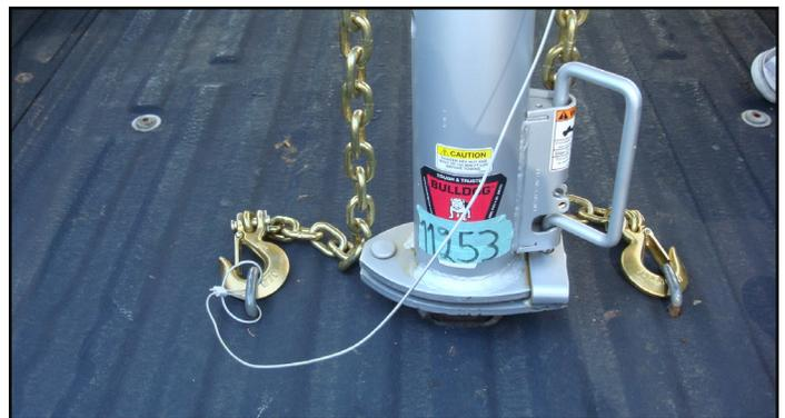
Fig.16 Safety Chain Arrangement
