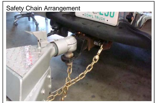
Visually inspect the safety chains and hooks for wear or damage. Replace worn or damaged safety chains and hooks before towing.
